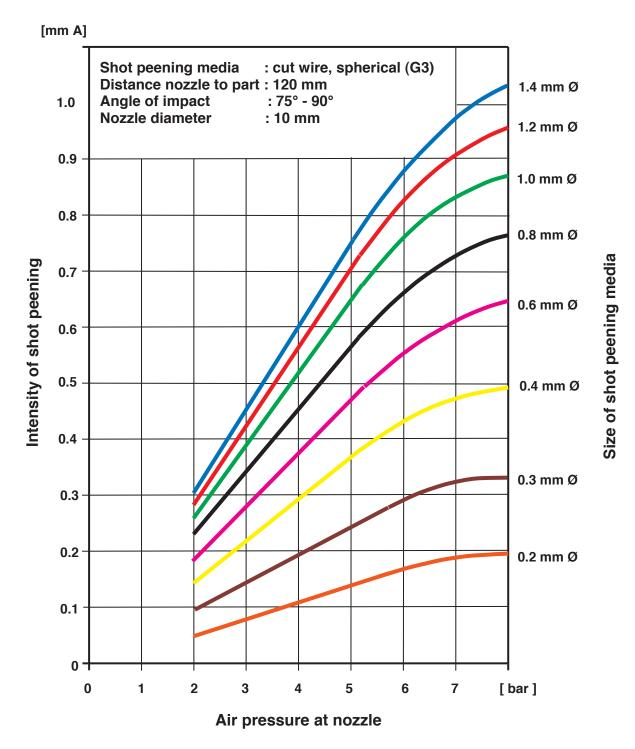
The necessary size of shot peening media to obtain the calculated depth of the compressive residual stress layer (see page 26) depends on the density and velocity of the shot peening media.
