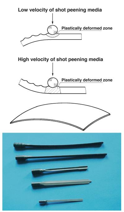
Air foils, wing surfaces, panels, sheets and other parts with relatively thin cross section, such as hardened rams, internal geared rings, etc., may be formed or straightened by shot peening within the elastic range of the material. If these parts are shot peened only on one side or selectively a convex curvature will be induced on the shot peened side.
