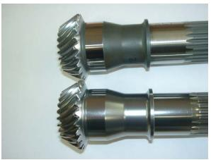
The surface finish of the tooth profile of gears can be improved by **vibratory grinding** after shot peening, because the process is indusing no temperature. But material removal should not exeed 10 % of the compressive stress layer.
